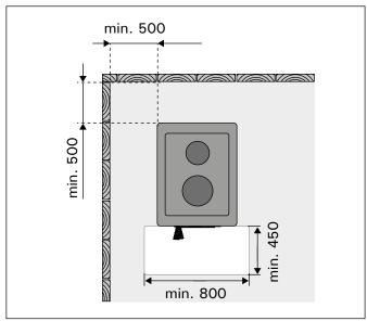
Figure 1. Safety distances (all dimensions in millimeters)
