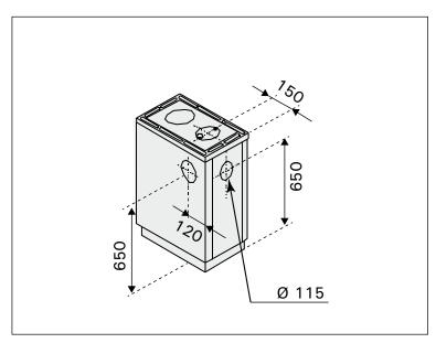
Figure 2. Location of smoke outlet (all dimensions in millimeters)
