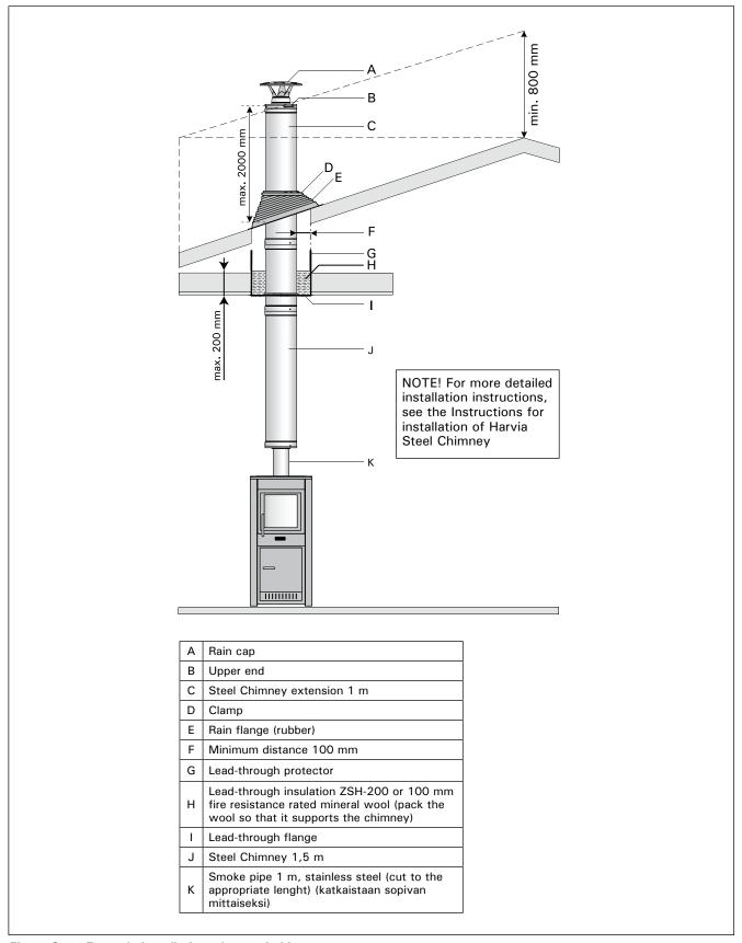
Figure 3. Example installation of a steel chimney
