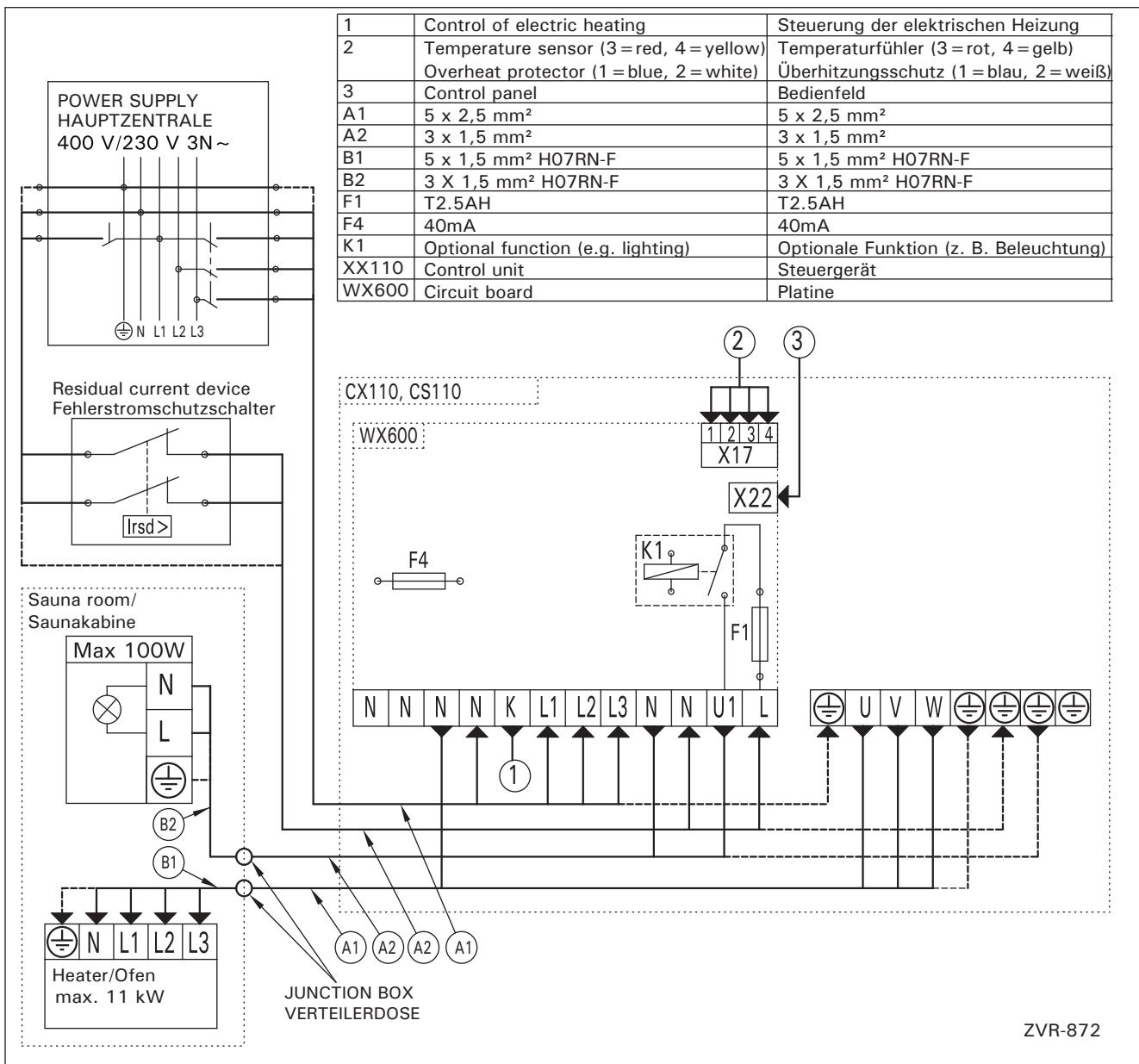
Figure 4. Electrical connections
