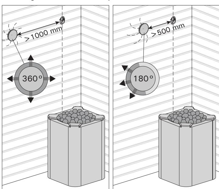
**Figure 7.** Sensor's minimum distance from an air vent
