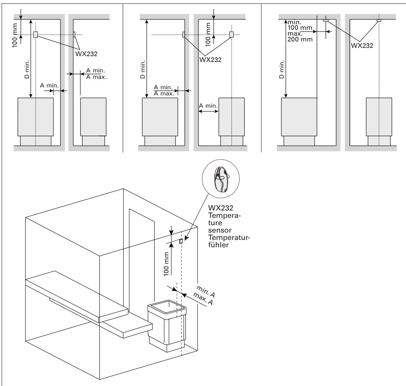
**Figure 6.** The place of the temperature sensor in connection with floor-mounted heaters
