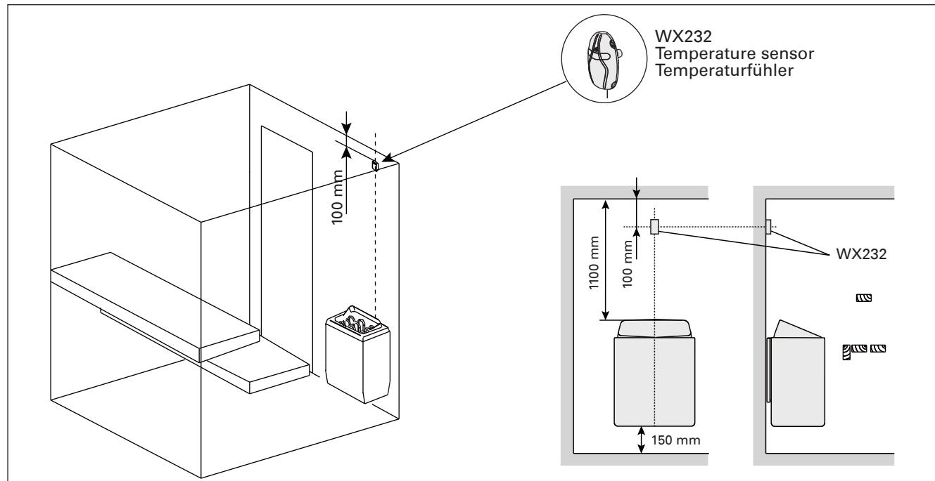
Figure 5. The place of the temperature sensor in connection with wall-mounted heaters
