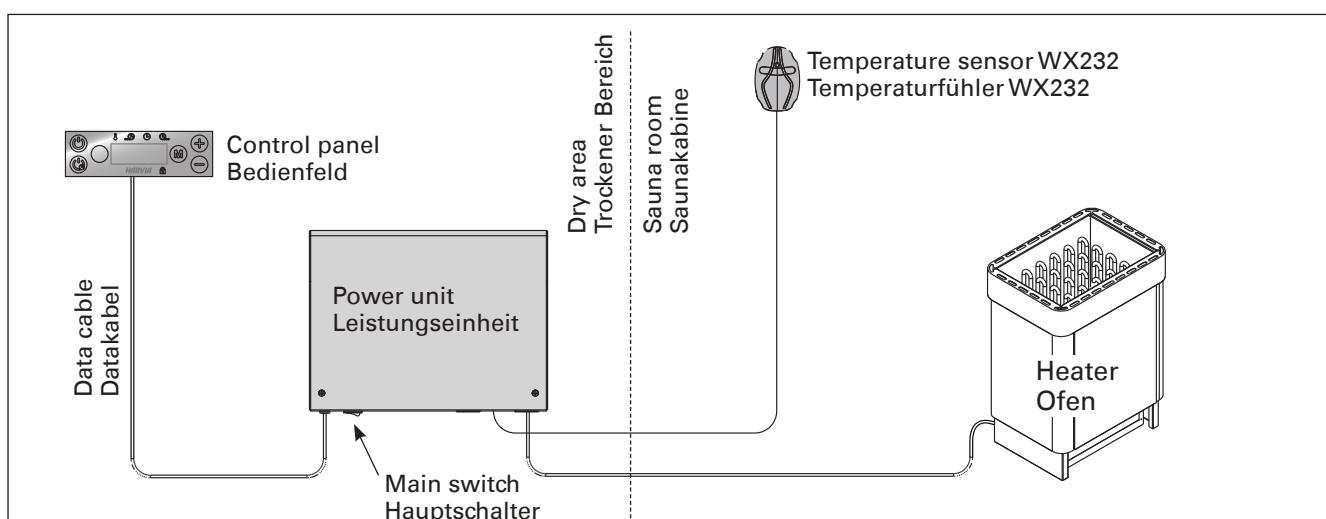
**Figure 1. System components**
