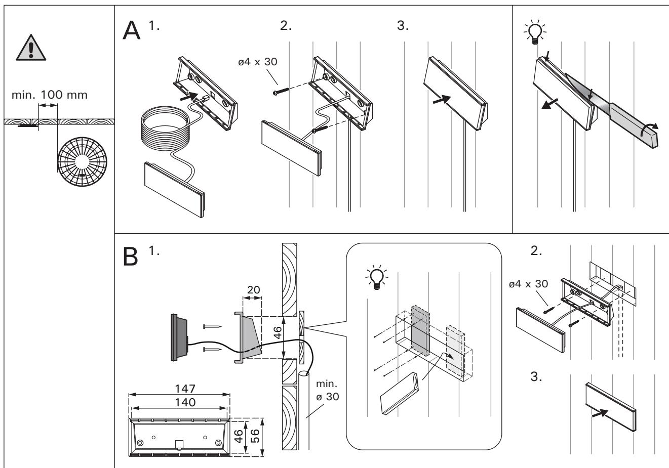
**Figure 2. Fastening the control panel**
