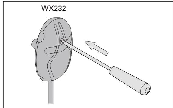
Figure 9. Reset button of the overheat protector
