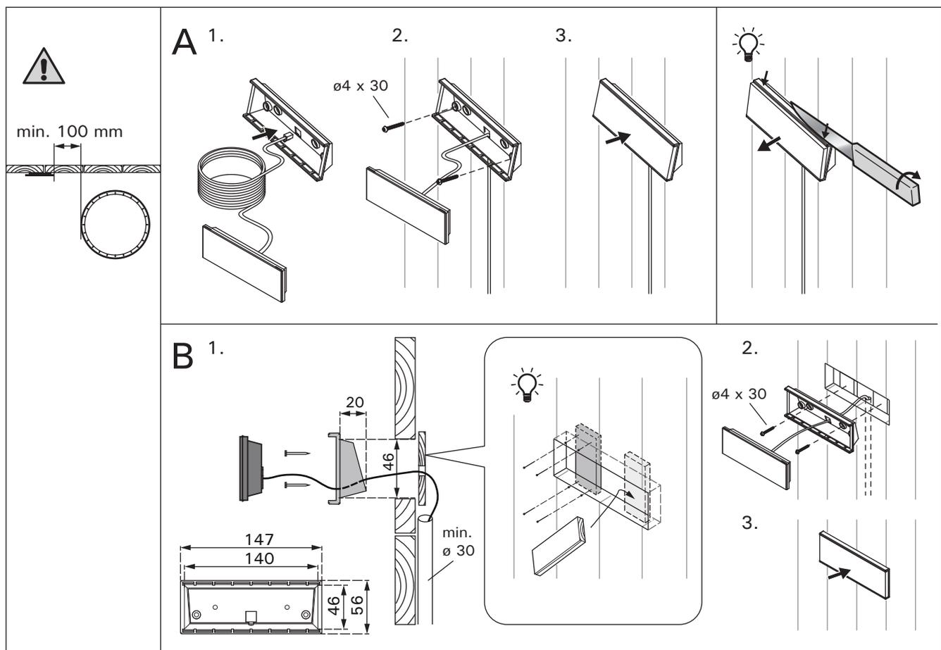
Figure 2. Fastening the control panel
