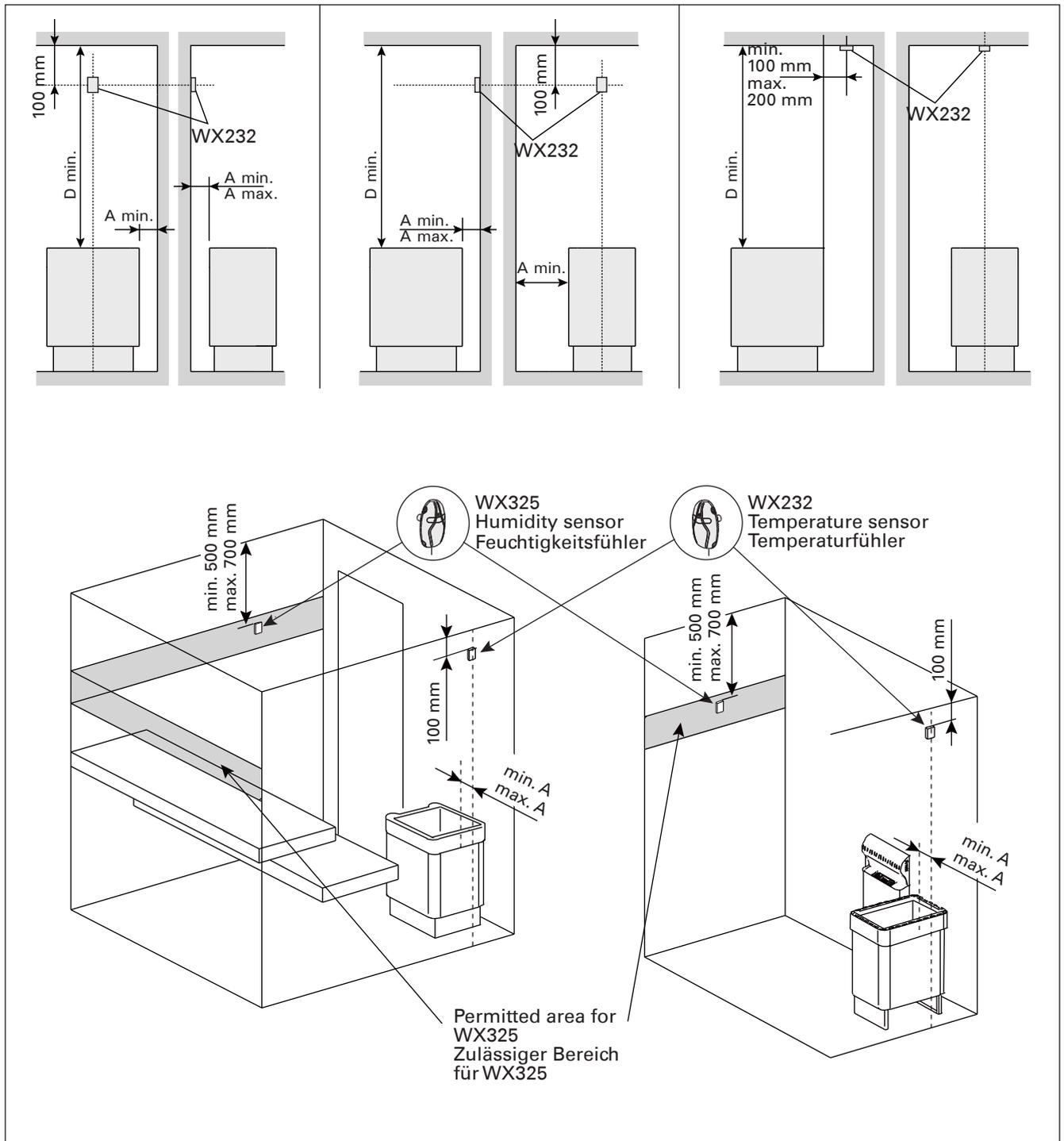
Figure 7. The place of the temperature and humidity sensors in connection with floor-mounted heaters
