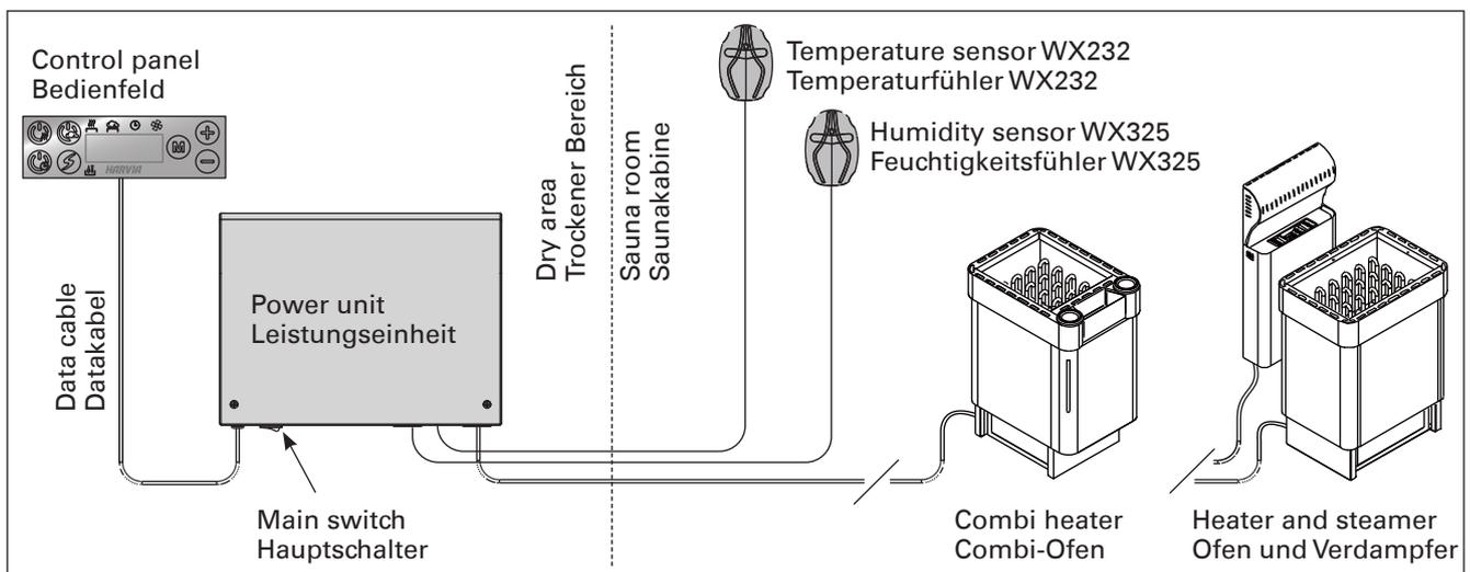
Figure 1. System components
