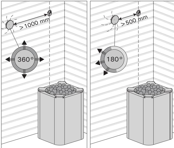
Figure 8. Sensor's minimum distance from an air vent
