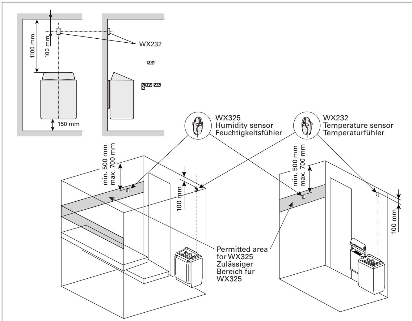
Figure 6. The place of the temperature and humidity sensors in connection with wall-mounted heaters
