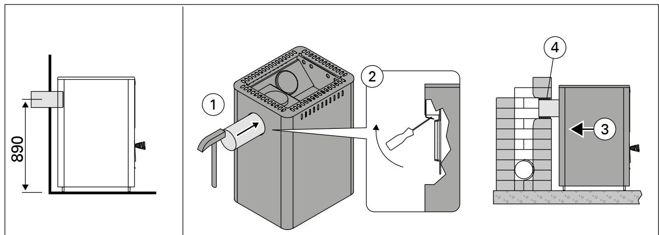
**Figure 8. Connecting the stove to a masonry flue via the rear connection opening (all dimensions in millimeters)**
