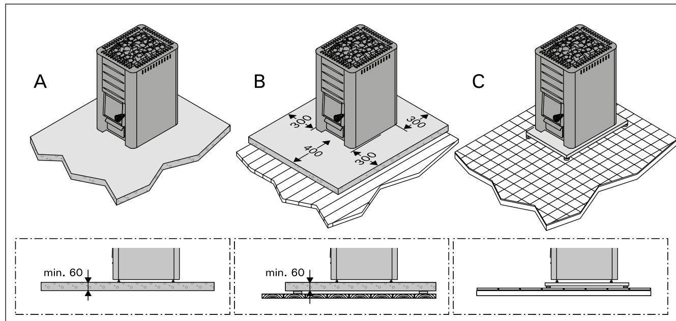
Figure 5. Protecting the floor (all dimensions in millimeters)
