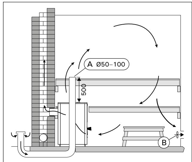
Figure 4. Mechanical exhaust ventilation
