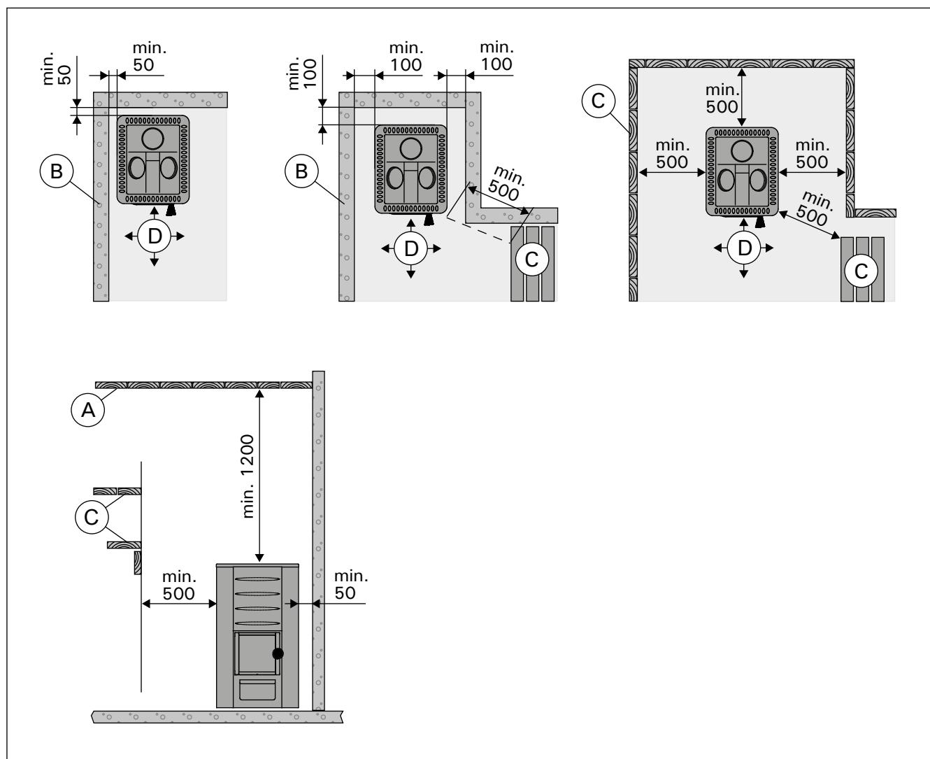
Figure 6. Safety distances (all dimensions in millimeters)
