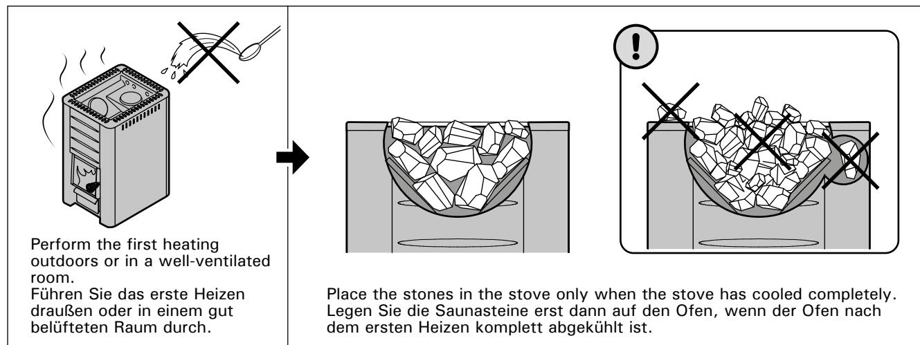
**Figure 2. Preparing the stove and piling the stones**
