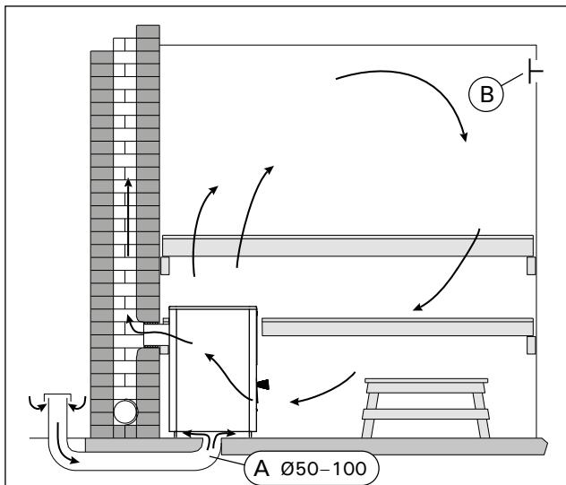
Figure 3. Gravity exhaust ventilation
