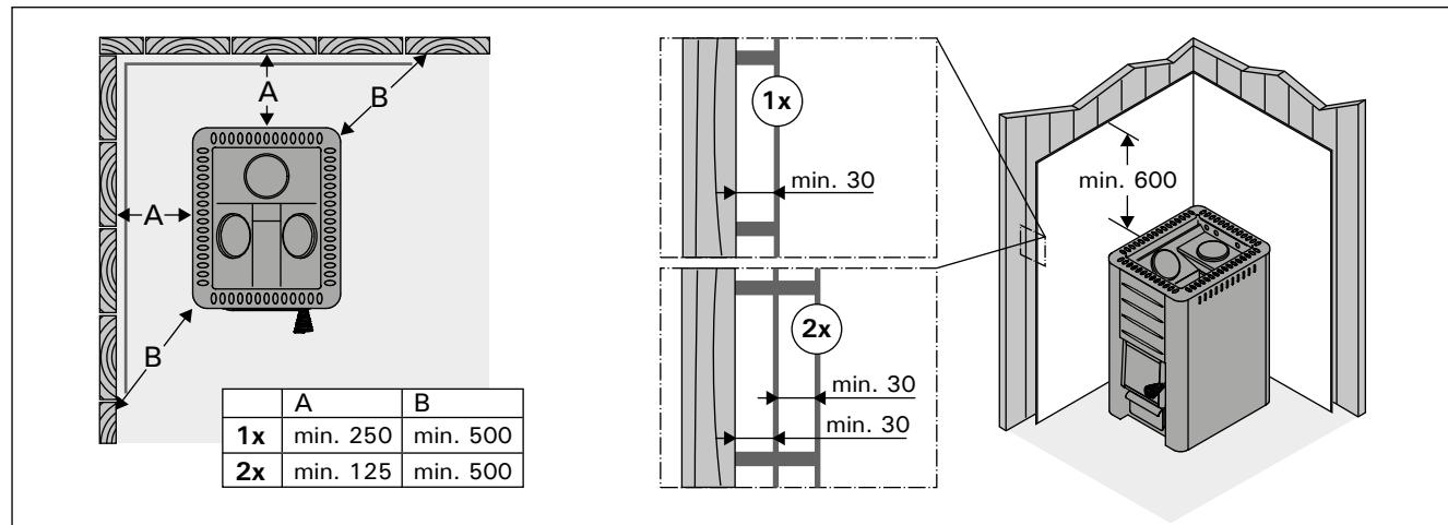
Figure 7. Protective covers (all dimensions in millimeters)
