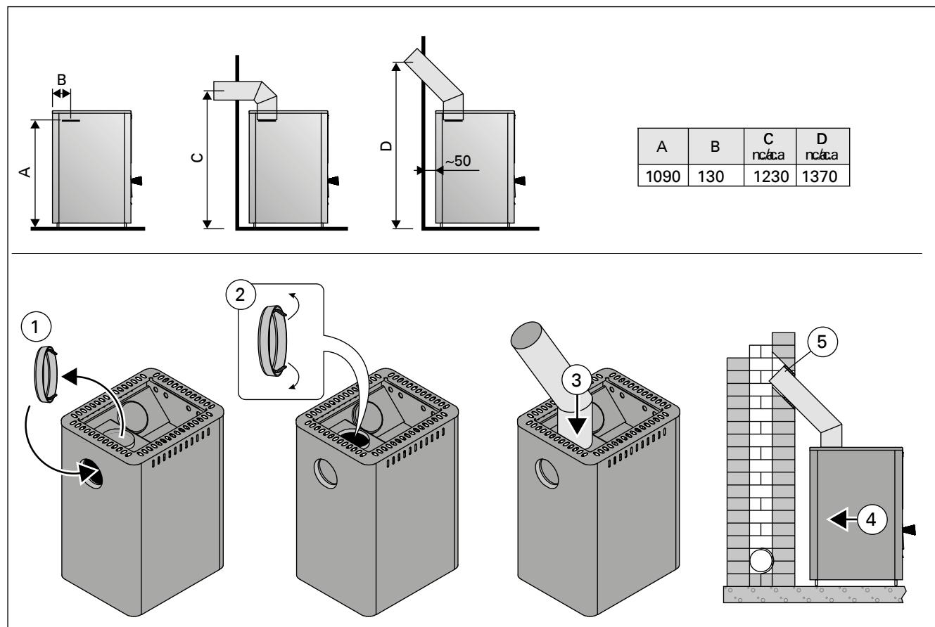
**Figure 9. Connecting the stove to a masonry flue via the upper connection opening (all dimensions in millimeters)**
